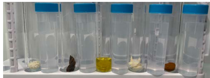
Figure 3. Samples Pre and Post Digestion (After Dilution). L to R: Instant Rice, Beef Jerky, Olive Oil, Mayo, Ground Turmeric
